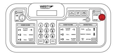
Pressing the **Set Clock** key on the keypad will take you to the **Set Clock Menu**. This menu will enable you to manipulate the scoreboard's clock. Use the **Up** and **Down** keys to scroll through several different options, listed below (for scoreboards with
